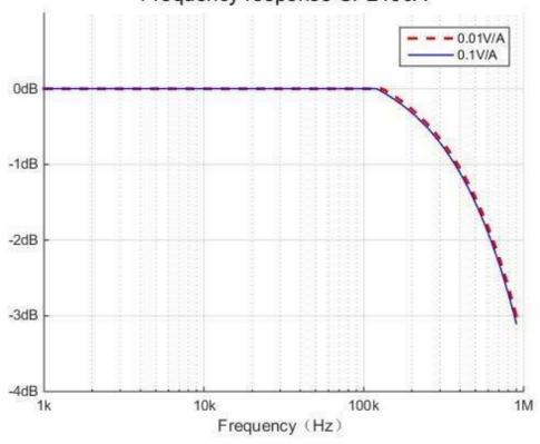
Amplitude-frequency characteristic curve -CP2100A
