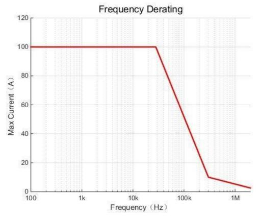
Maximum current versus frequency Frequency response CP2100A
