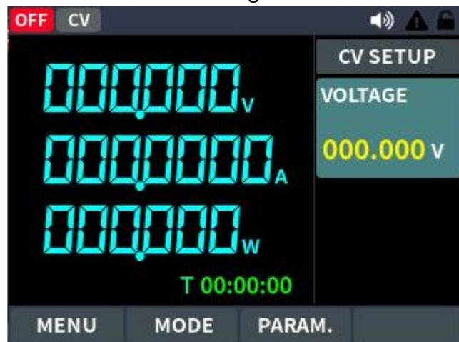
Figure 4.3.2-2 CV mode operation interface
