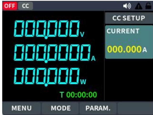
Figure 4.3.1-2 CC mode operation interface
