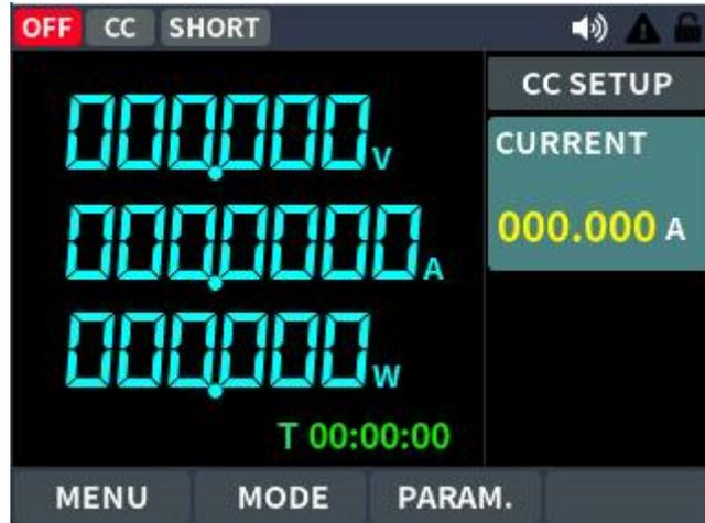
Figure 4.6-1 Short circuit simulation interface
