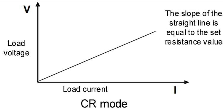
Figure 4.3.3-1 CR mode: The Voltage-Current Relationship Diagram
