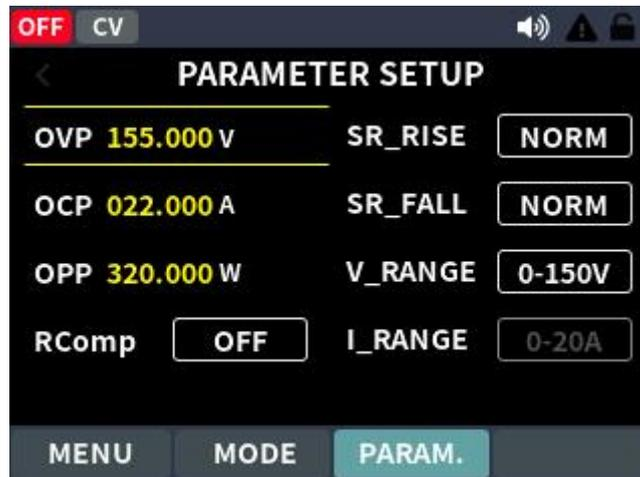
Figure 4-7-2 parameters setup page
