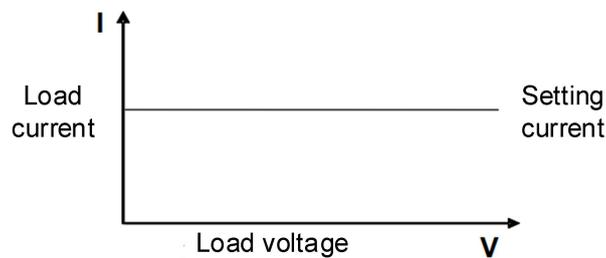
Figure 4.3.1-1 CC mode: The Voltage-Current Relationship Diagram
