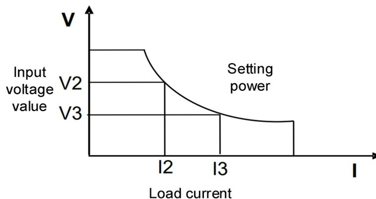
Figure 4.3.4-1 CP mode: The Voltage-Current Relationship Diagram
