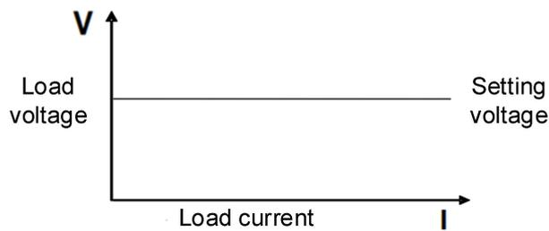
Figure 4.3.2-1 CV mode: The Voltage-Current Relationship Diagram
