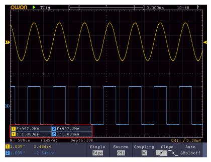
Figure 4-13 Automatic measurement
