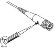
Figure 3-8 Adjust Probe
