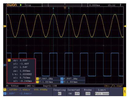
Figure 4-16 Time&Voltage Cursor Measurement
