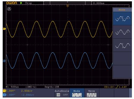
Figure 4-17 Autoscale Horizontal-Vertical multi-period waveforms
