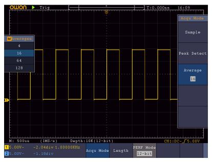
Figure 6-5 Reduce Noise level by using Average function
