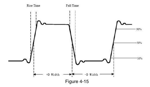
Figure 4-15 shows a pulse with some of the time measurement points.
