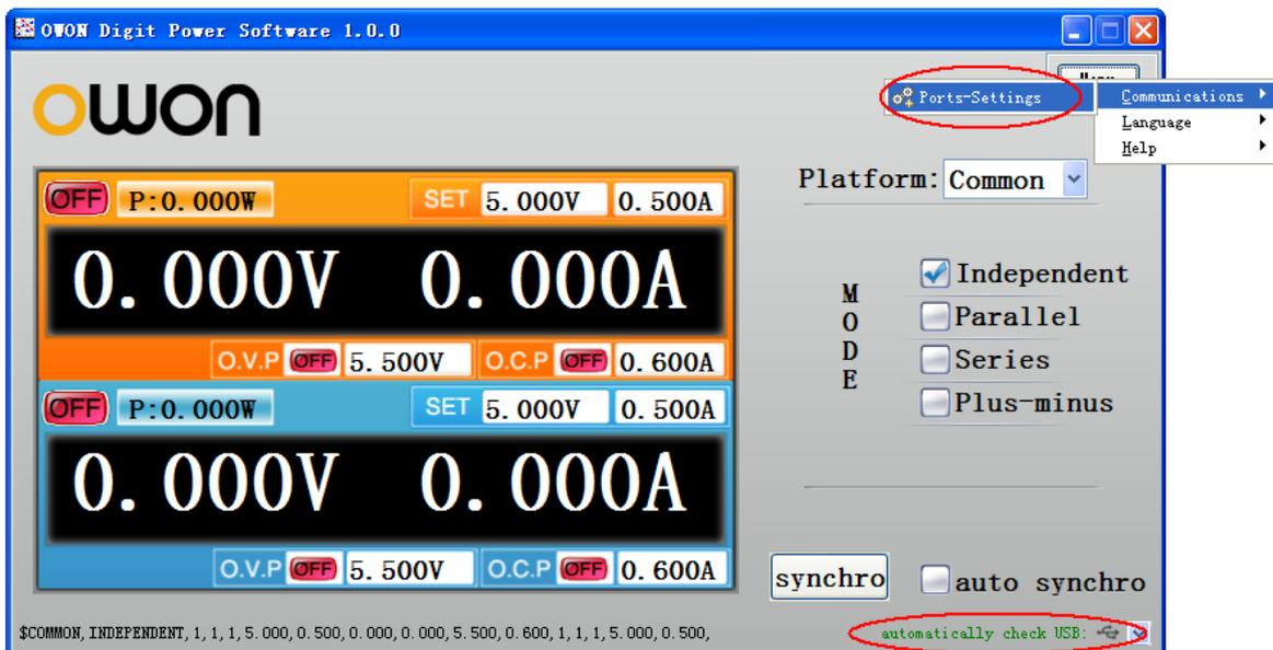
Figure 6-1: The Power Supply connects with PC successfully
